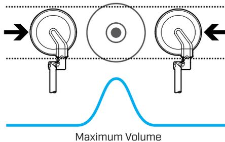
Figure 22: Determine target centre
