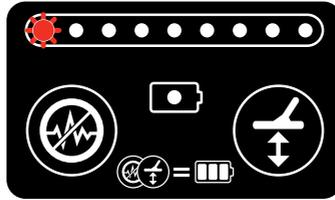
Figure 11: LED Display with no target response
