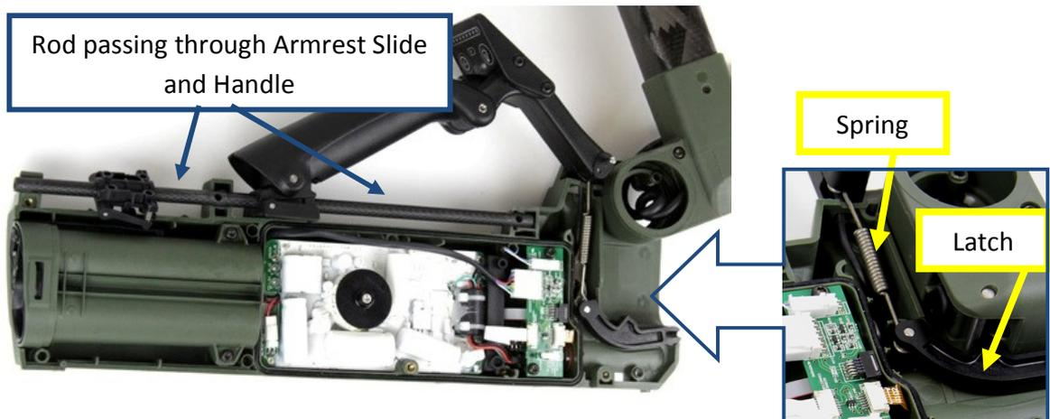
Figure 84: Latch Hinge and Spring Latch Hinge
