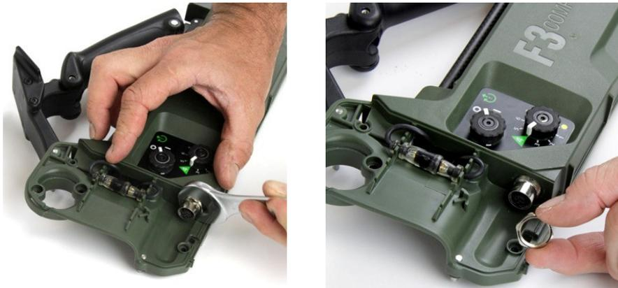
Figure 32: Removing the Coil Connector Nut (18mm)
