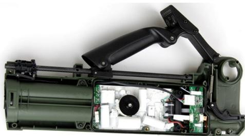
Figure 91: Opened Detector Body
