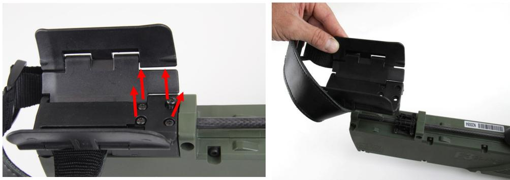
Figure 9: Removing the Armrest
