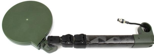
*Figure 74: Shaft and Coil Removed from Detector*
