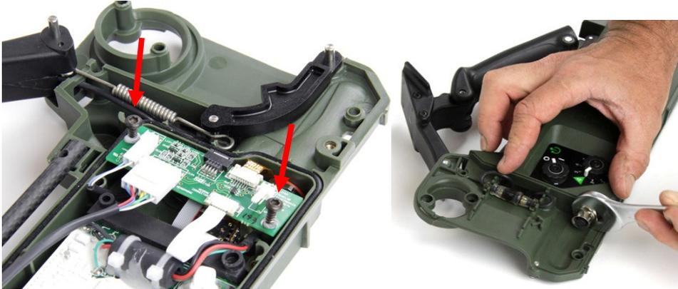
*Figure 46: Interface PCB and Coil Connector Nut*
