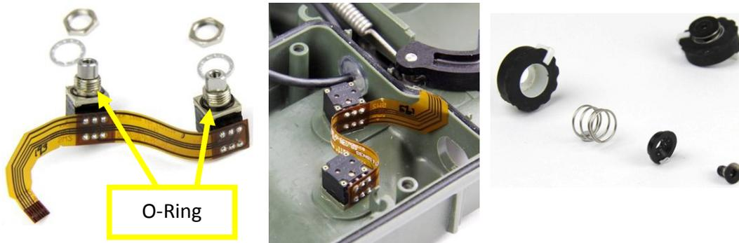
Figure 94: Control Switches
