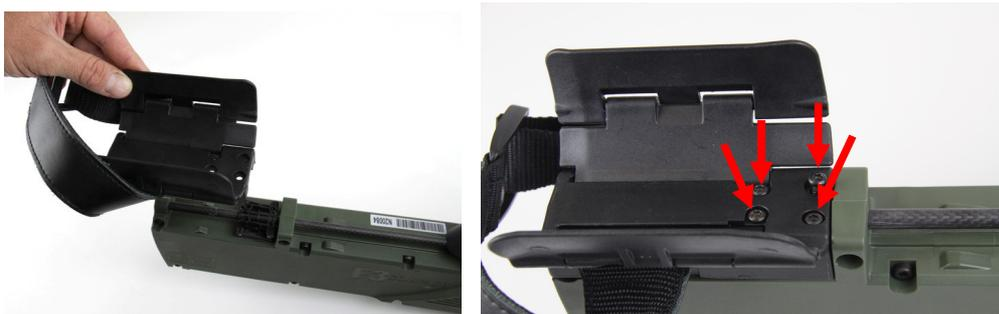
Figure 28: Attaching the Armrest
