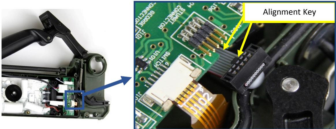
Figure 43: Connector 10 Way
