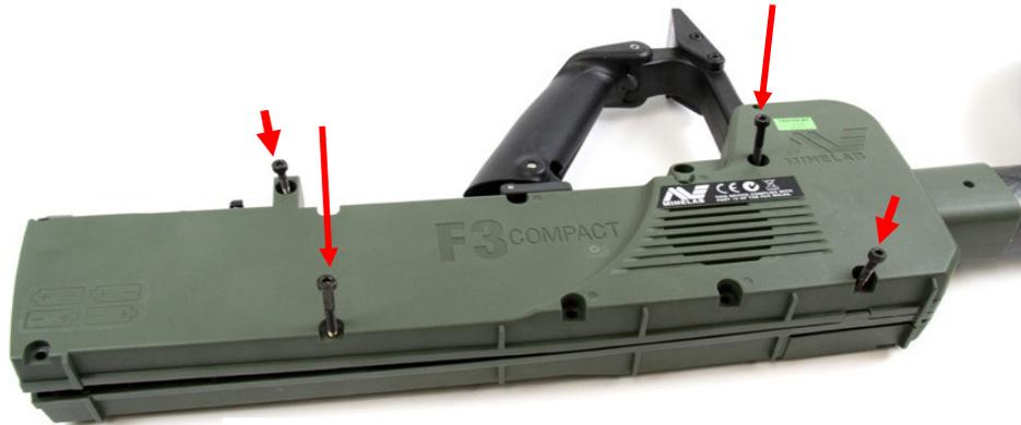
Figure 22: Fitting Four Screws
