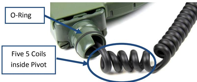
Figure 60: O-Ring and Coil Cable
