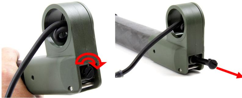
*Figure 75: Removing Pin Coil Cable*
