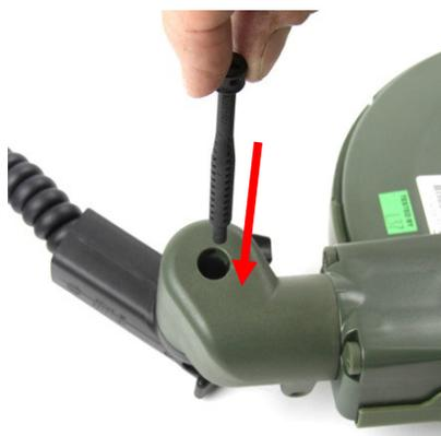
Figure 63: Inserting Pin Coil Pivot
