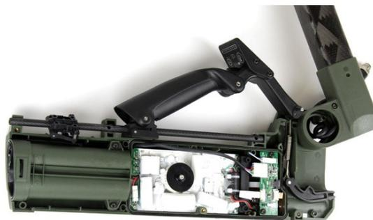
Figure 69: Connecting Shaft and Coil
