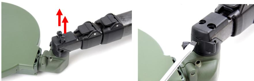
Figure 52: Removing Screws from Lower Shaft
