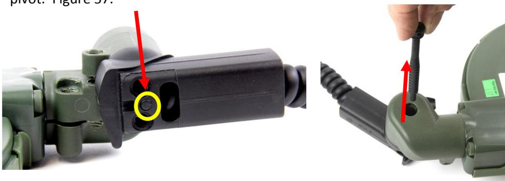
Figure 57: Removing Pin Coil Pivot
