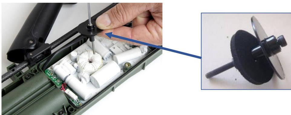
Figure 42: Screw Toroid
