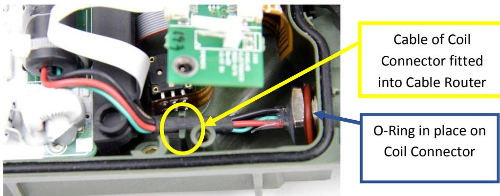
Figure 41: Coil Connector
