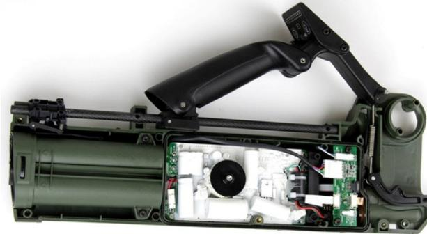
Figure 31: Opened Detector Body
