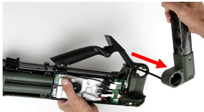
*Figure 15: Removing Shafts*
