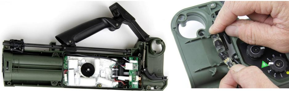
Figure 80: Disconnect Wiring Loom Handle
