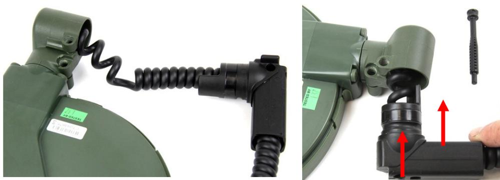
Figure 62: Fitting Pivot Lower Shaft
