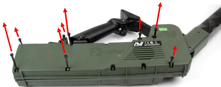
Figure 12: Removing 8 Screws.
