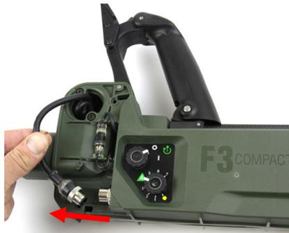
Figure 50: Disconnecting Coil Connector
