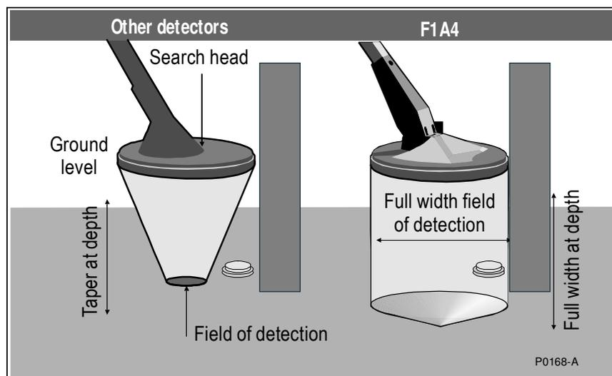
***Minelab has detection that covers the entire width of the search head. This means that deminers have less chance of missing mines while they are demining (CMAC Trial Report 1998)***
