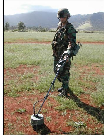
The HSTAMIDS project (due for completion in 2004) seeks to replace the existing fleet of US Army hand held detectors with state of the art dual sensor (ground penetration radar and metal detection) technology. Over the past three years, Minelab has continued to develop its metal detection technology as part of its contribution to this high profile project.
